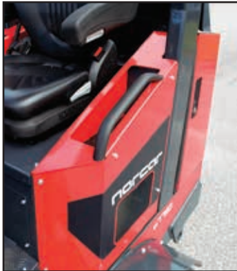
Handle for safe and easy access to driving seat. Storage boxes on both sides for tools, phone and accessories. 12V and USB outlets.
