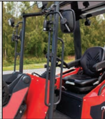
Handle for safe and easy access to driving seat. Storage boxes on both sides for tools, phone and accessories. 12V and USB outlets.
